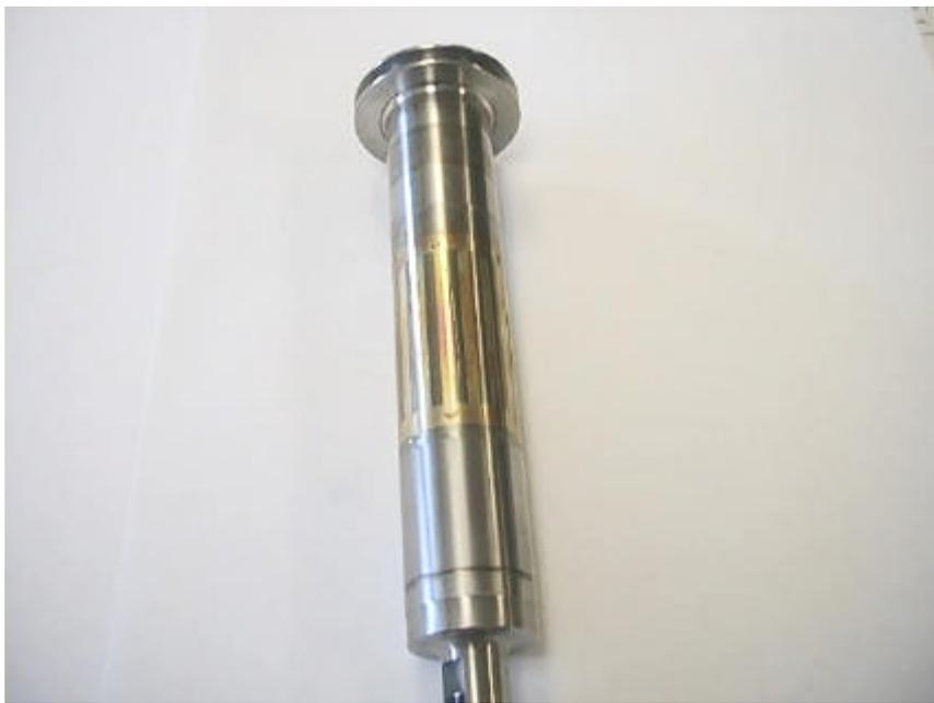
The parts pictured above show the damage sustained during operation and seizure of the spindle.
